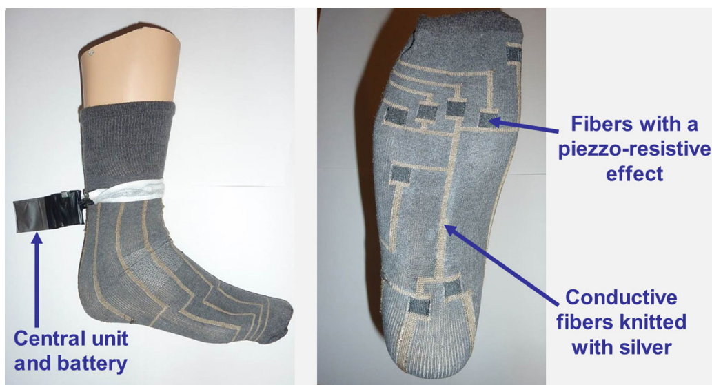
Fig. 2. The sock knitted with fibers coated with silver (current conduction) and with fibers having a piezo-resistive effect. The central unit (left) is connected to the silver-coated fibers and to a soft battery.
