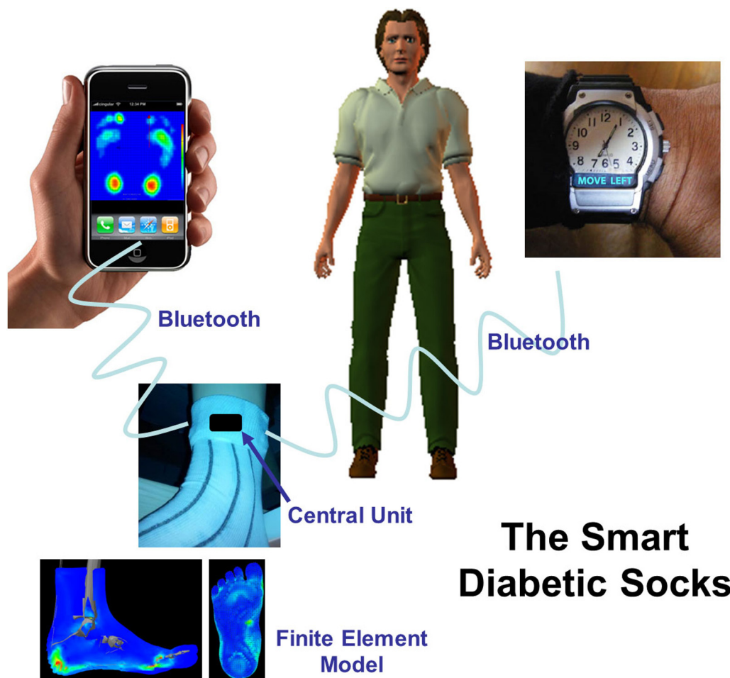
Fig. 1. Framework for the Smart Diabetic Socks device.
